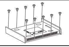
Remove the 8 M4 screws from the screen frame and remove the screen frame.
