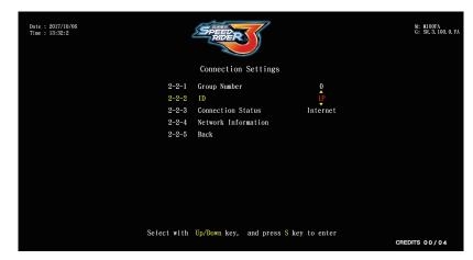
You can use the [Up], [Down] keys to select [Network Information], press to enter the page, then check MAC Address, IP Address, Subnet Mask, Gateway are all correct.
