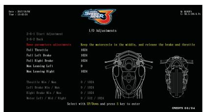
4 Under the [Full Throttle] option, fill up the throttle and press the skey to move on to the next reset option. Each option will have a corresponding image.
