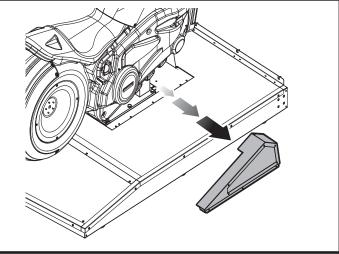
Remove the 2 M4 nuts and the light bar holder beneath the vehicle.
