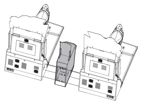
**1** Open coin box back door, and secure the 1p and 2p with 8 M6 screws.
