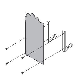
**5** Secure the middle cardboard and card description support bracket with 4 M4 screws
