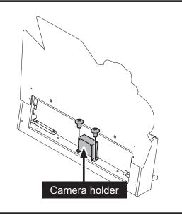
Remove the 11 M4 screws, Billboard maintenance door, and camera holder.
