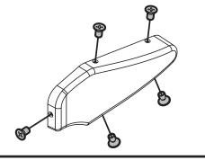
Replace the light bars and reassemble according to the reversed assembly sequence.
