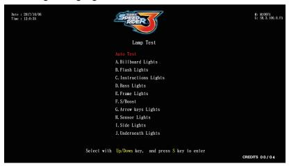
If you want to test a certain light: Use the [Up],[Down] to choose the items and press the button, and the tested light will keep blinking. Press the button to discontinue your testing.
