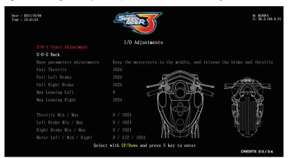
3 When the cursor is pointing to [Base parameters adjustments], then keep the motorcycle in the middle position, releasing the brake and throttle. Then press Sbutton.
