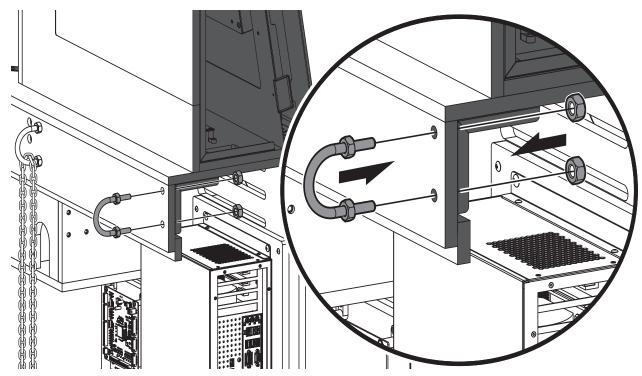
① Open the maintenance door and then secure U-shaped hook with screws from the inner side.
