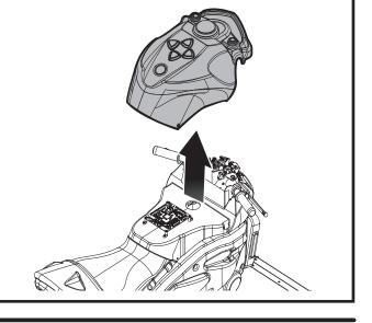
Remove the 4 M3 screws, replace the infrared sensor circuit board, and reassemble according to the reversed assembly sequence.
