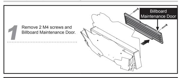
Then remove the 8 M2 screws, replace the light bar, and reassemble according to the reversed assembly sequence.
