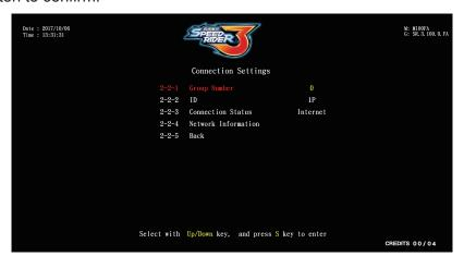
**3** Setting the ID of the main cabinet: Select the ID by using [Up] and [Down] buttons. Then press the Sobutton to confirm.
