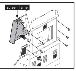
Remove the 10 M4 screws from the screen frame.
