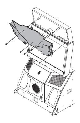
3 Secure the assembled LOGO acrylic and screen holder with 2 M4 screws and 4 mirror bead screws.
