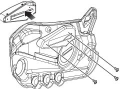
Remove the 5 M4 screws from the side panel light cover.
