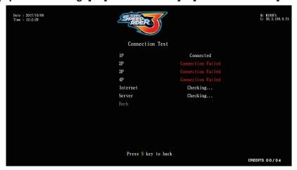
2 In the page of [Connection Test], press the button, and the system will start sending the connection status of all cabinets. Possible connection status includes:
