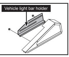
Replace the light bars and reassemble according to the reversed assembly sequence.
